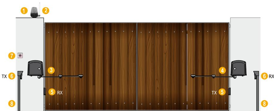
1\_Flashing light 2\_Outstanding antenna 3\_LH operator featuring control board and radio receiver
