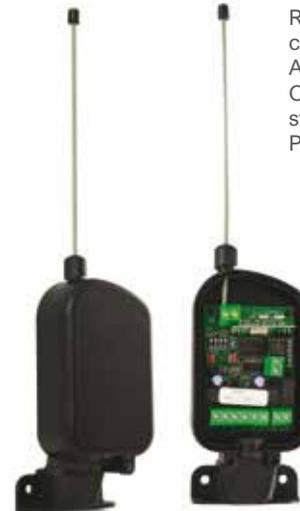
Radio receiver for external mounting, complete with case and aerial. Available in 1 or 4-channel version. Optional memory card with 512 code storage capacity. Power supply 12/24V ac/dc.
